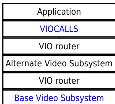
OS/2 Video subsystem placed in VIOCALS.DLL. Called VIO function passes control to internal VIO router function which, depends on registered functions replacement, routes call to Base Video Subsystem (BVSCALLS.DLL) or to registered Alternate Video Subsystem.
