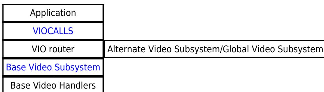
OS/2 Video subsystem placed in VIOCALS.DLL by default (or some another place for other OSes). Called VIO function passes control to VIO router function which, depends on registered functions replacement, routes call to Base Video Subsystem (BVSCALLS.DLL) or to registered Alternate Video Subsystem. Base Video Subsystem utilises Base Video Handlers (BVH\*.DLL). Base Vide Handler is a sort of video hardware abstraction layer.
