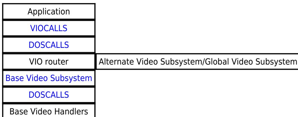
OS/2 Video Subsystem is 16-bit. Later three independed versions of 32-to-16 bit wrapper subsystems was developed (See Fig)
